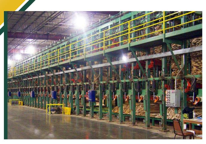
**TS Manufacturing offers a variety of Bin Sorting Systems customized to suit your application**. Systems range from the proven pusher lug or drag chain systems, to automatic lumber cart filling and chop line sorting bins.
