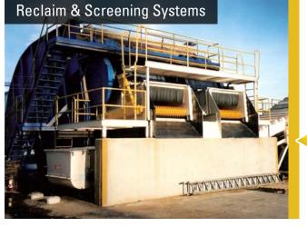
These systems allow a large amount of material to be efficiently stored and metered into your boiler system. These can be fed by Truck Dumping Systems (available with integrated screening), or Loader Systems, depending on requirements. Reclaims are available in truck receiving, multi-chain or belt style systems.
