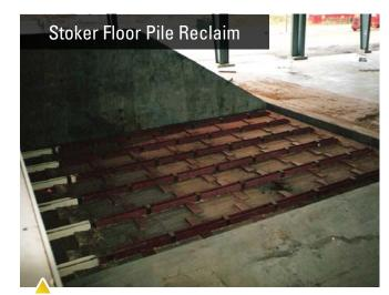
Stoker Floor Reclaims offer the many benefits pile reclaiming, with minimal maintenance. These 'Stoker Floor' or 'Ladder Floor' systems can sustain enormous piles in covered or open air environments. With the addition of a dust shroud and lump breaker, these systems allow increased uptime and flexible pile sizes. Their rugged construction allows the size of the pile to be significantly larger than the active floor area. Driving on top of the floor system, for pile reshaping, is common.
