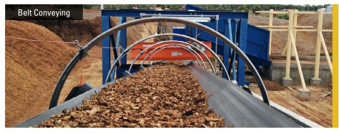
TS Belt Conveyors are available in trough, flat slider and tube conveyor designs. Our adjustable skirting ensures a smooth transition of materials and prolongs belt life. Impact sections are custom engineered to suit your application. Optional hoods keep elements out of the material and dust in.
