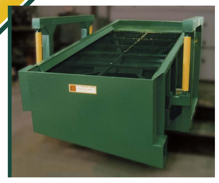
TS Rotary Screens are available in standard sizes ranging from 12 to 66 units\*. Their counter-balanced design allows for high speed operations and lower equipment fatigue. The durable construction incorporates tie rod mounting and heavy duty, double taper, roller bearings for maximum durability and reduced maintenance.
