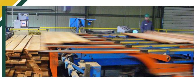
TS Manufacturing Stackers are custom designed for specific applications, and incorporate our 40+ years of lumber handling knowledge. Our Lumber Stackers are available in electric or hydraulic models - based on customer request. Their simple, rugged design is built to meet the most demanding hardwood and softwood applications with high flexibility and precision.
