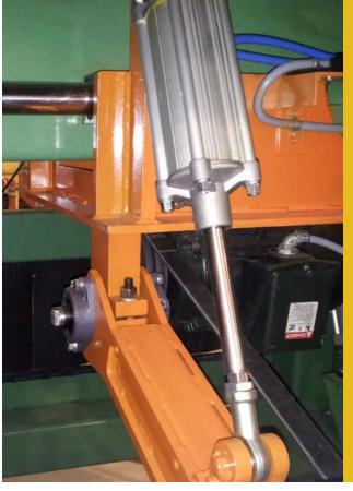
For raisable saw systems, the cylinder and belts are identical to the rest of the trimmer for interchangeability.
