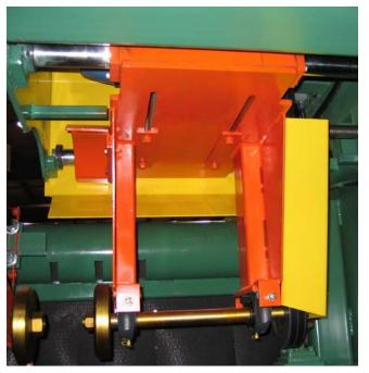
An available feature of the TS Lineshaft Trimmer is the mini-adjustable 0' end lineshaft. This system is becoming more popular as the drive for efficiency necessitates ever more flexible solutions.
