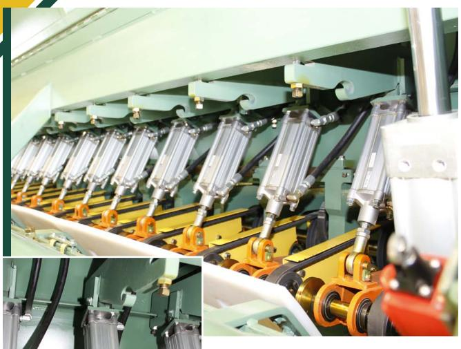
Modular design in the TS Lineshaft Trimmer allows for the flexibility to meet demanding length specifications. The pictured 1' saw spacing still provides rapid access for all belt and saw changes.
