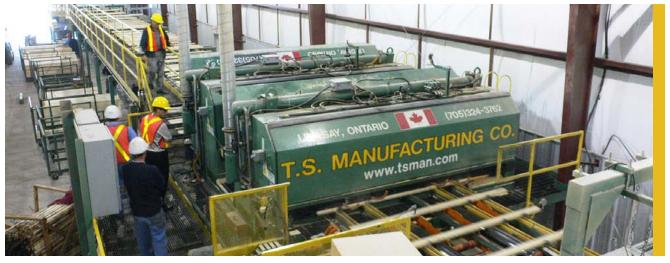
Each TS Trimmer is provided with an integrated 'gull wing' door system, (including pneumatically operated doors and safety bar), ensuring the system can be safely accessed when the pneumatics are isolated.
